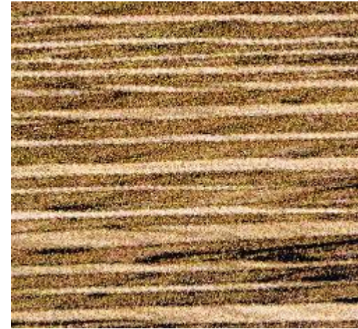
Stripe domains in nematic elastomer Kundler & Finkelmann Mathematical theory due to De Simone & Dolzmann
