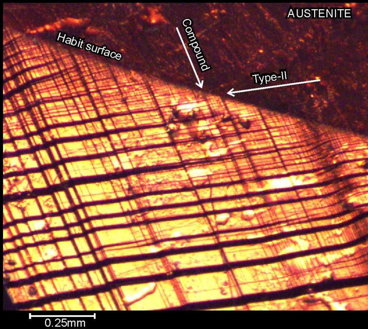
Optical micrograph (H. Seiner) of non-classical interface between austenite and a martensitic microstructure
