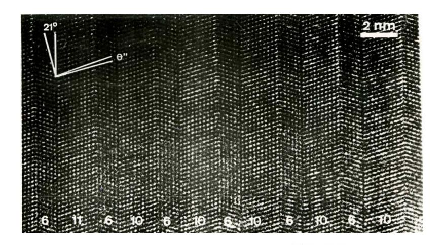
Atomistically sharp interfaces for cubic to tetragonal transformation in NiMn
