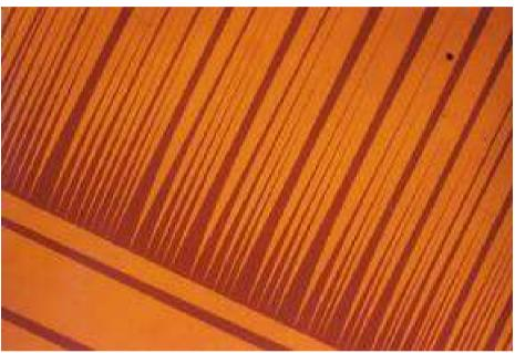
Interfaces correspond to pairs of matrices A, B with  $A - B = a \otimes N$ , where N is the interface normal. At minimum energy  $A, B \in K(\theta)$ .
