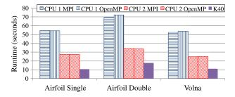
Figure 5. Baseline performance on Airfoil, in single precision and double precision (2.8M cell mesh), and Volna in single precision (2.4M cell mesh).
