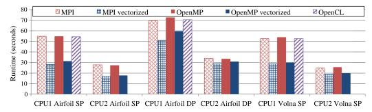
Figure 6. Vectorization with explicit vector intrinsics and OpenCL, performance results from Airfoil in single (SP) and double (DP) precision on the 2.8M cell mesh and from Volna in single precision on CPU 1 and 2.
