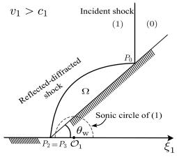
**Figure 19.** The attached subsonic regular reflection-diffraction configuration [6].
