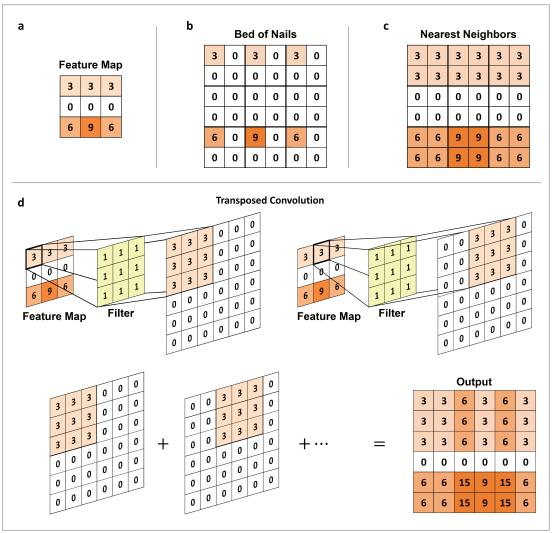
**Figure 5.** Examples of upsampling a single (a) feature map using (b) bed of nails, (c) nearest neighbors, and (d) transposed convolutions. The transposed convolution is performed using a 3x3x1 filter and a stride of two. Note the weights within the transposed convolutional filters are learned from the data during CNN training.
