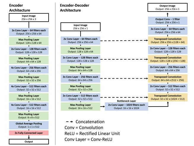
**Figure 6.** *Prototypical encoder and encoder-decoder architectures.* Encoder networks (left) map an input image to a 1D space, which is ideal for classification and regression tasks. Encoder-decoder networks (right) map an input image to another image by first encoding the input image onto a lower-dimensional space (bottleneck layer) and then upsampling the bottleneck feature maps back to image space.
