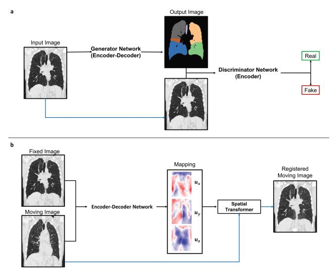
**Figure 8.** (a) Image-to-image translation GAN and (b) CNN-based registration framework. The pix2pix GAN is often used to synthetize images to supplement training. In the registration framework, an encoder-decoder architecture is trained to predict a spatial transformation represented by a vector field (i.e., mapping) that is used to map the moving image to fixed image space.
