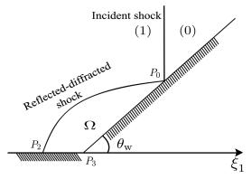
**Figure 17.** Subsonic regular reflection-diffraction configuration [6].
