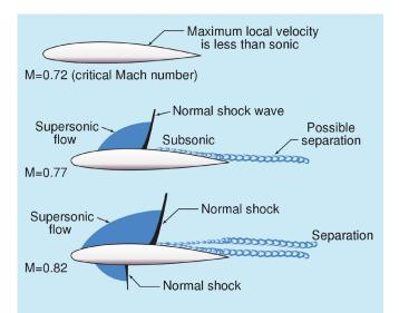
**Figure 10.** Transonic flow patterns on an airfoil showing flow patterns at and above the critical Mach number.
