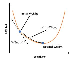
**Figure 9.** Illustration of the gradient-descent optimization algorithm. Prior to network training, weights are randomly initialized. The gradient of the predetermined loss function is then calculated with respect to the weights and evaluated for each training observation. Weights are adjusted by the product of the gradient and a preselected step size  $\gamma$ . The process is iteratively performed until the loss is minimized or stops improving.
