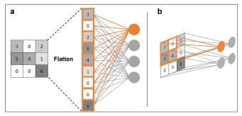
**Figure 2.** Difference between (a) fully-connected networks and (b) CNNs when applied to images. Fully-connected networks require images to be flattened prior to being propagated through the network. Each neuron is connected via a weight to every neuron in the prior layer. In a CNN, each neuron is connected to a small area on the input image; output neurons are arranged in a manner that preserves spatial information.
