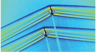
Figure 3. NASA's first Schlieren photo of shock waves interacting between two aircraft (taken in March 2019).
