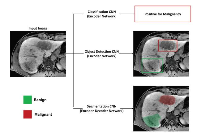
**Figure 7.** *Diagram showing the differences between commonly performed medical imaging tasks.* Classification categorizes the entire input image into a set of finite classes. Object detection identifies objects within an image, localizes the objects using a bounding box, and determines the class of the object within the same architecture. Segmentation partitions an image into meaningful classes at the pixel level, which can be used to calculate anatomical measurements, such as lesion size.
