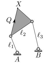
Figure 2. Schematic of a four-bar linkage.
