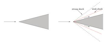
**Figure 7.** Two steady solutions with shocks around the solid wedge with an angle  $\theta_{w} \in (0, \theta_{w}^{s})$  or even  $\theta_{w} \in [\theta_{w}^{s}, \theta_{w}^{d})$ .
