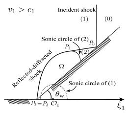
**Figure 18.** The attached supersonic regular reflection-diffraction configuration [6].
