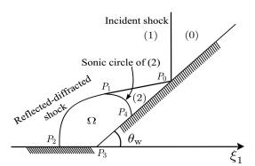
**Figure 16.** Supersonic regular reflection-diffraction configuration [6].
