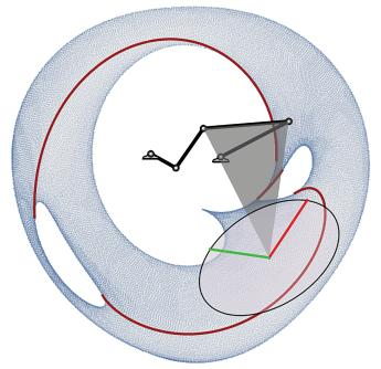
**Figure 3.** Workspace curve of input singularities and velocity ellipse for a five-bar linkage.
