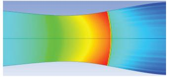
**Figure 4.** Diagram of a de Laval nozzle for the approximate flow velocity.
