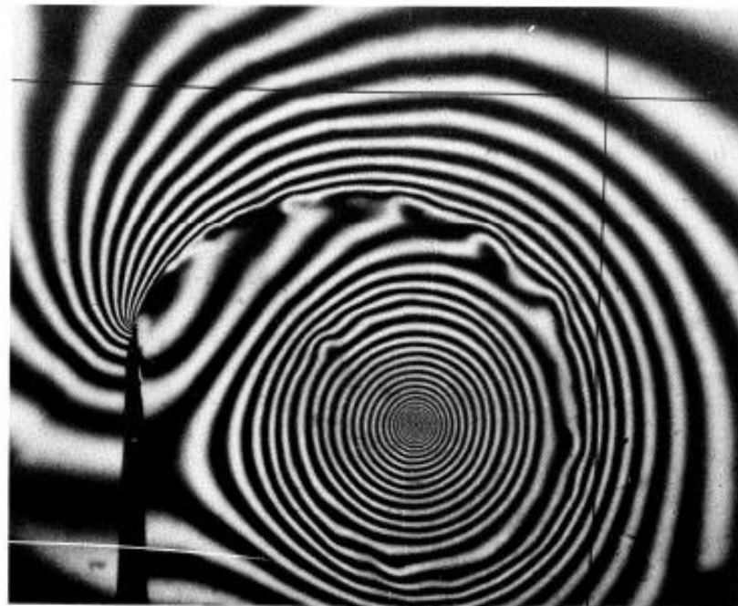
83. Density in a vortex from a wedge. A quite different view of the phenomenon above is given by this infinite-fringe interferogram, which shows lines of constant den-
