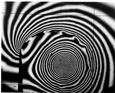
83. Density in a vortex from a wedge. A quite different view of the phenomenon above is given by this interference interferogram, which shows lines of constant density.
