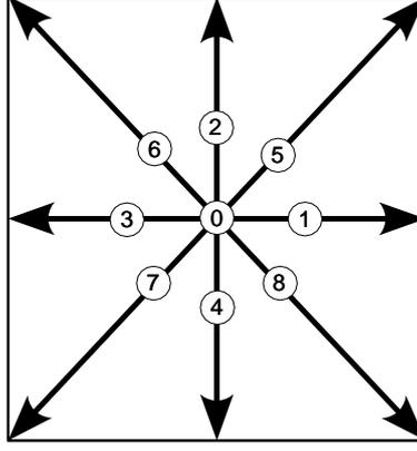
One may go from the partial differential equation Eq (3) to a lattice Boltzmann equation (1) by integrating along characteristics with the trapezium rule for a timestep  $\Delta t$ .
