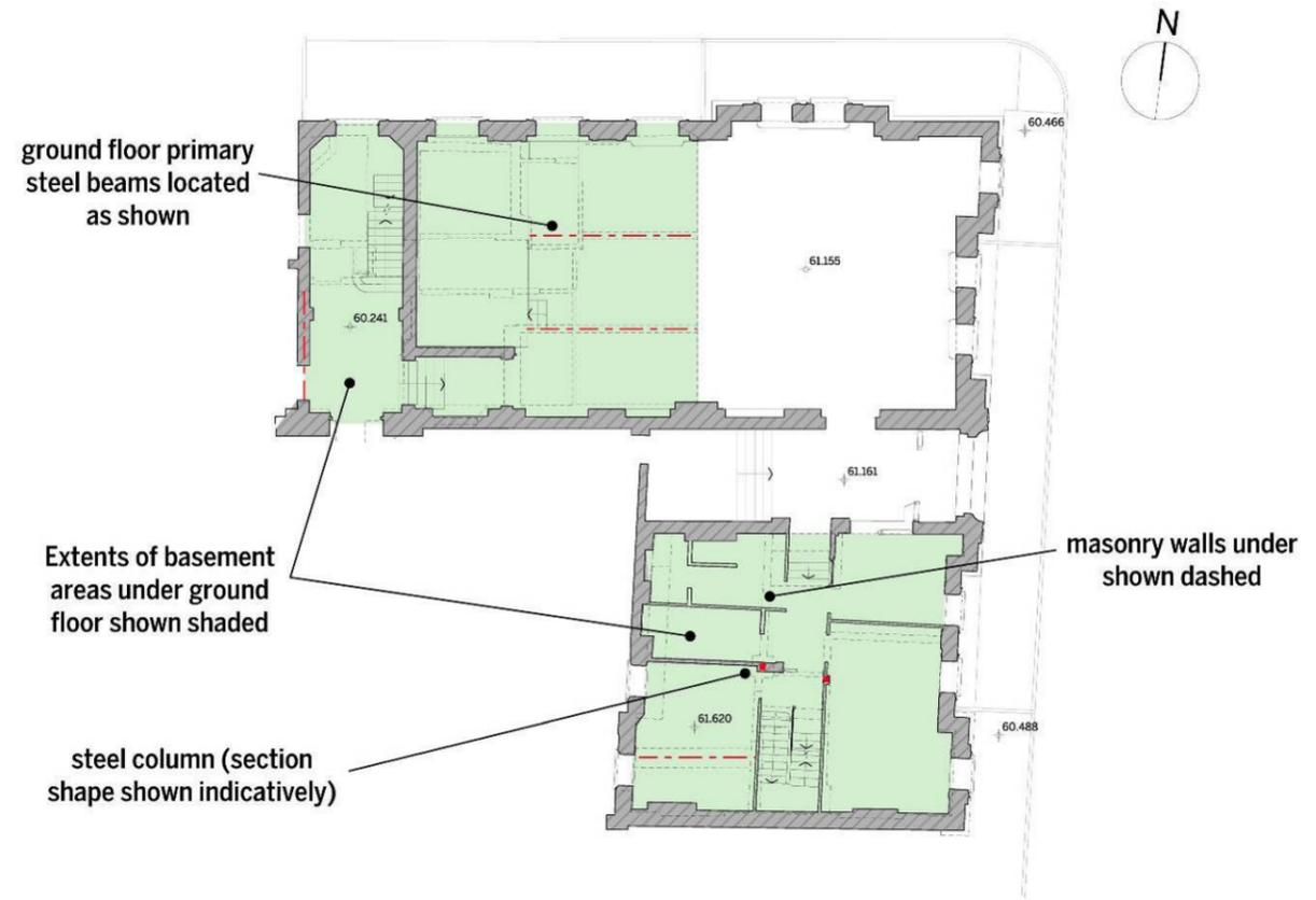
**Figure 4 Ground Floor Structural Arrangement**
