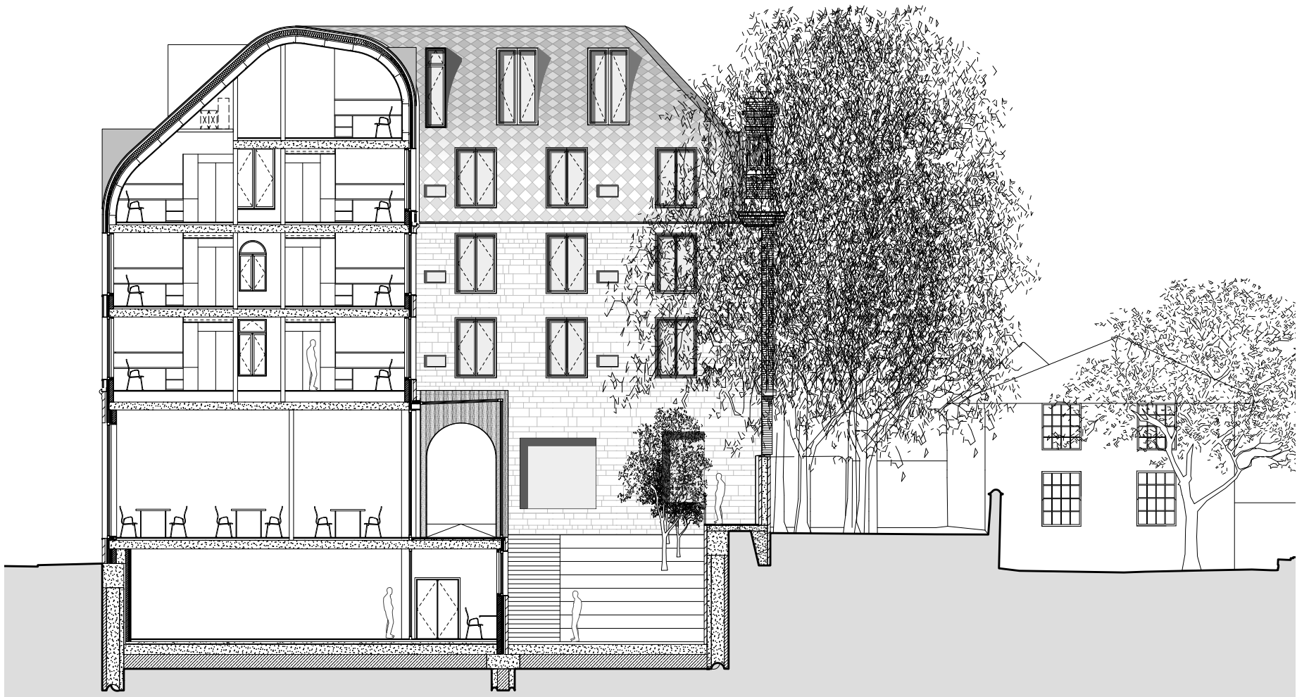
Section through retained Ruskin facade and proposed building
