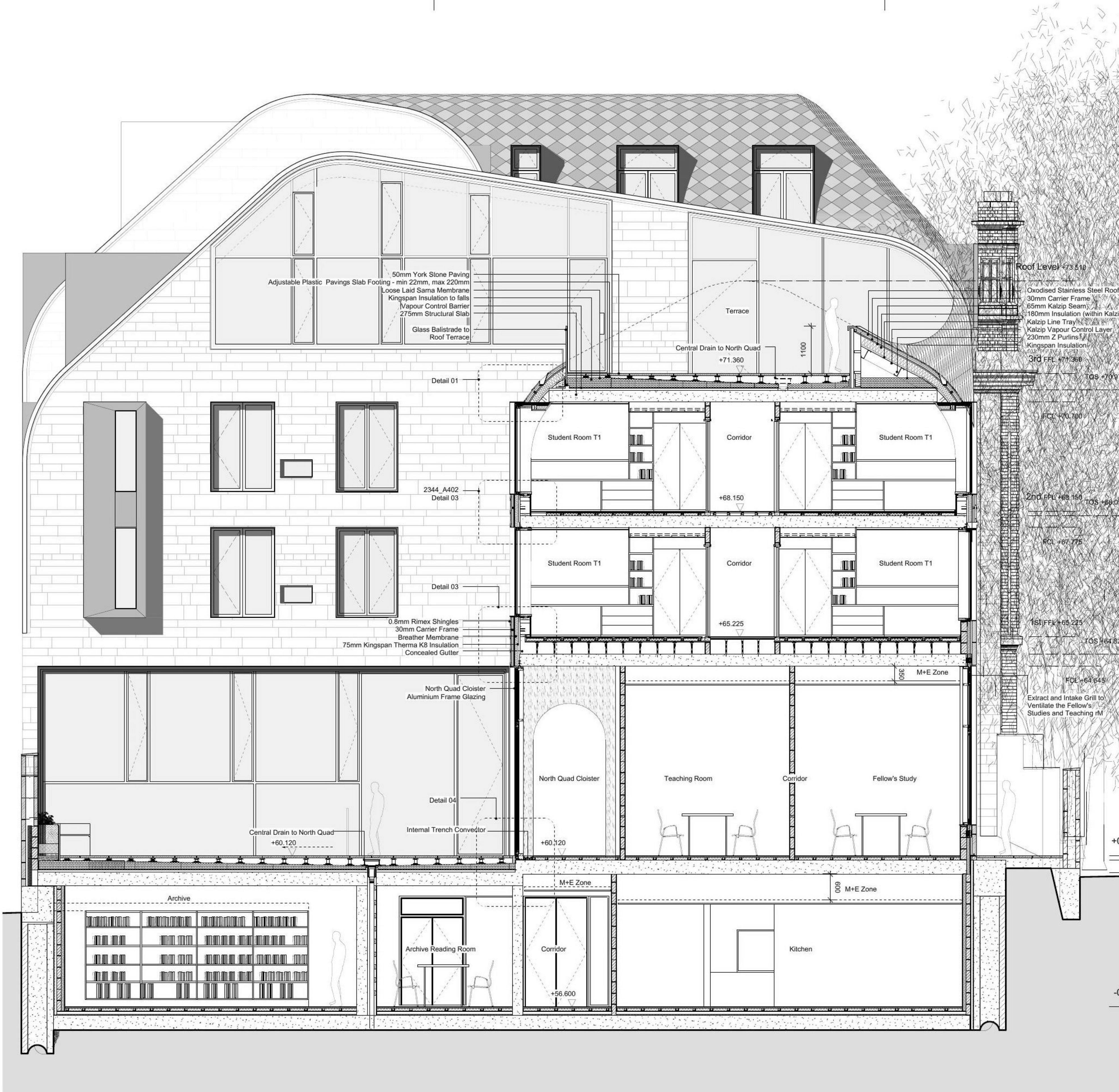
1 SECTION THROUGH WEST WING / NORTH QUAD
