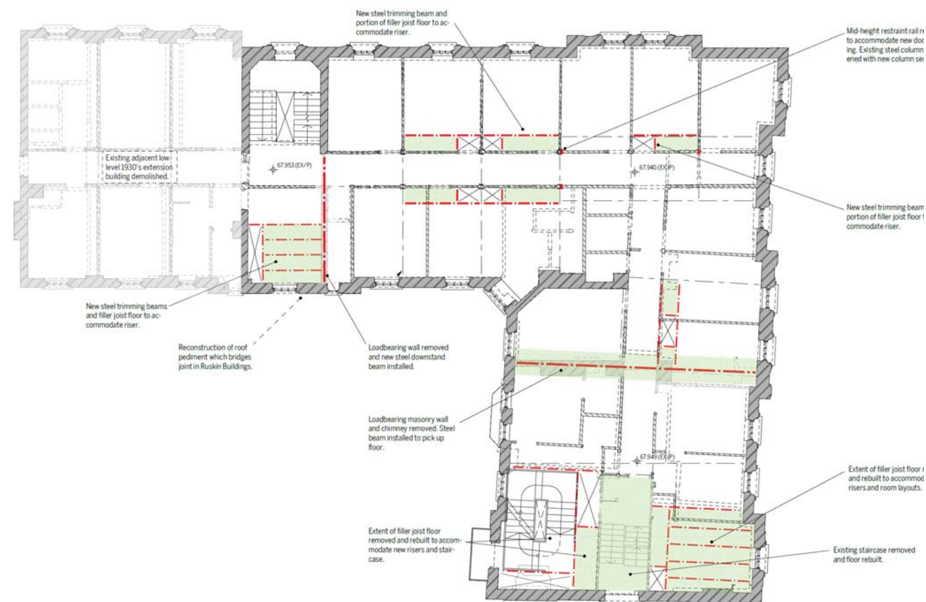
Figure 2: Ruskin Building Typical Upper Floor Intervention
