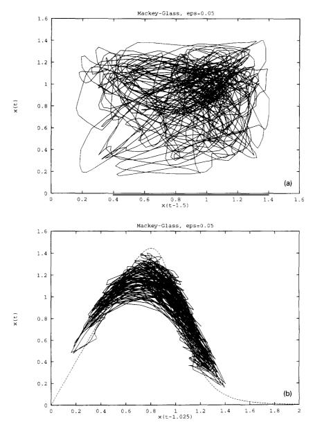
Fig. 5. Phase plot of fig. 1, x versus  $x_{\delta}$ : (a)  $\delta = 1.5$ ; (b)  $\delta = 1.025$ .
