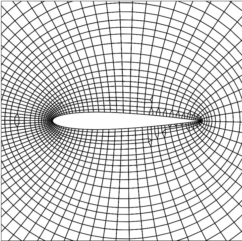
Figure 3: NACA0012; first coarsening
