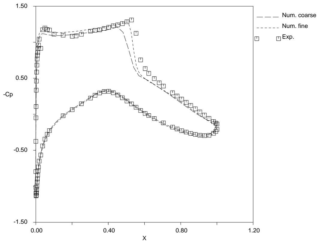
Figure 14: RAE2822; coefficient of pressure
