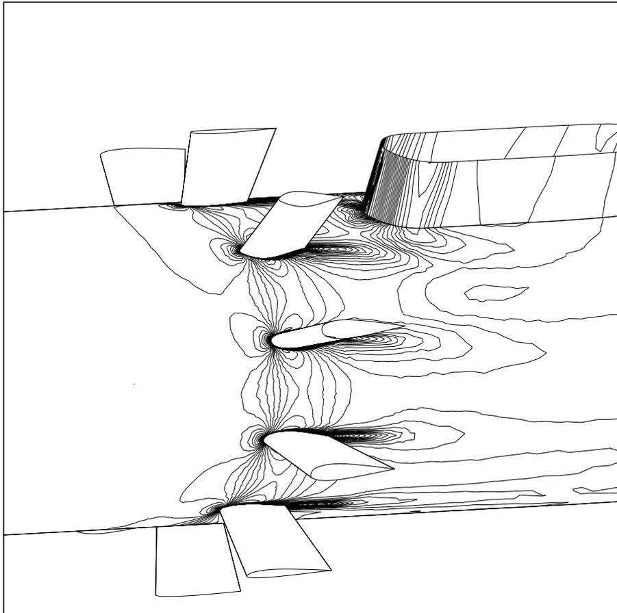
Figure 16: 3D Bypass duct; Mach number contours
