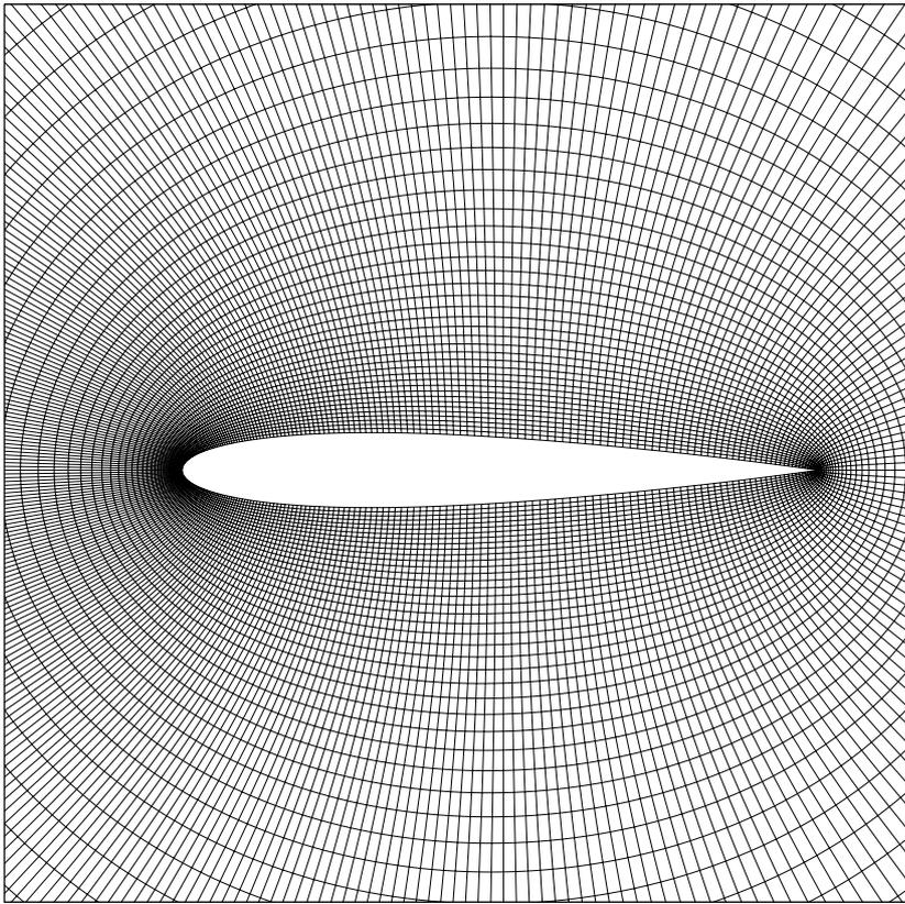
Figure 2: NACA0012; fine grid
