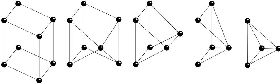
Figure 1: Collapsing edges on a hexahedron.
