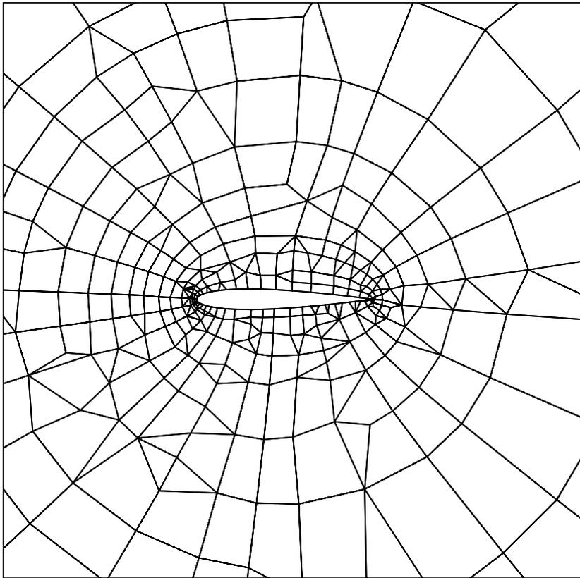
Figure 4: NACA0012; fourth coarsening
