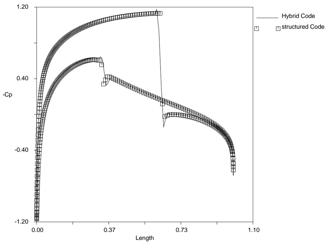
Figure 5: NACA0012; coefficient of pressure
