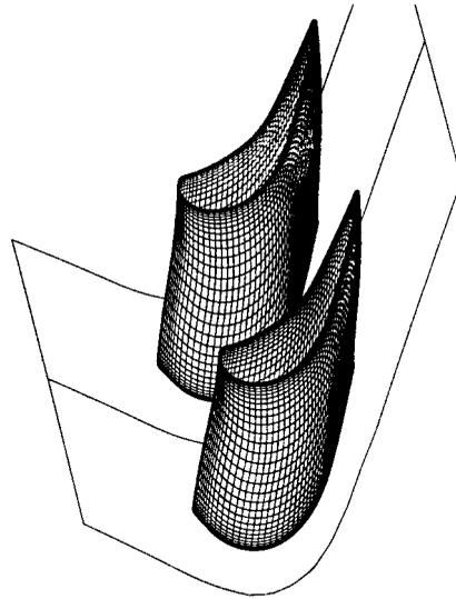
Figure 4. High pressure turbine geometry used for the example application.
