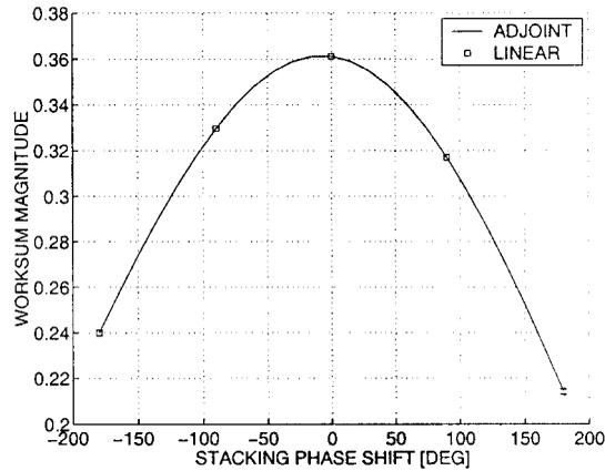
Figure 5. Worksum magnitude versus maximum re-stacking phase shift.
