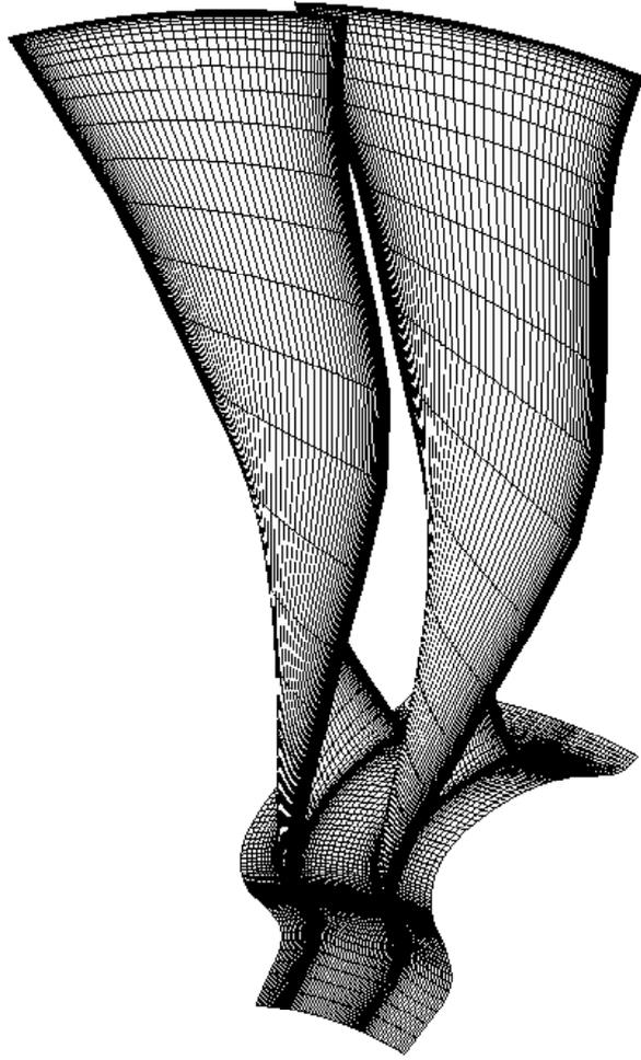
Figure 8: Blade geometry and surface mesh of the 3D fan.
