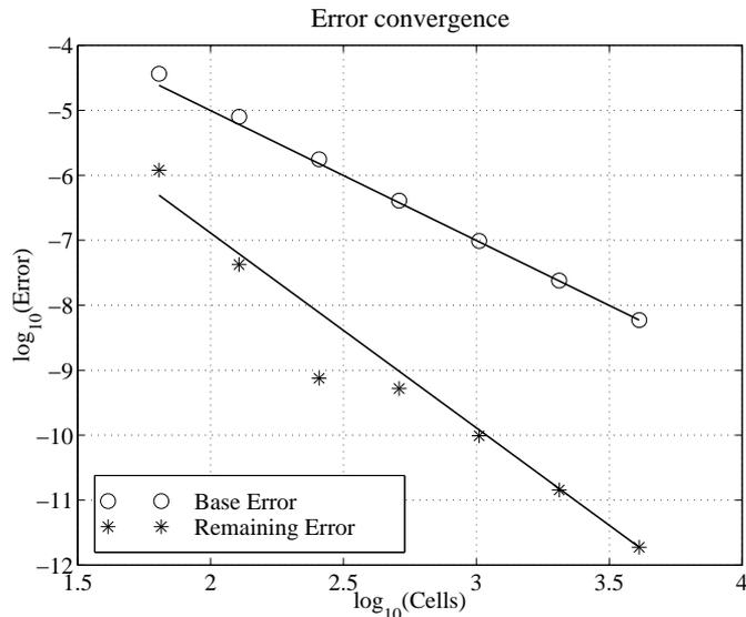
**Fig. 8.** Error convergence for quasi-1D shocked flow.
