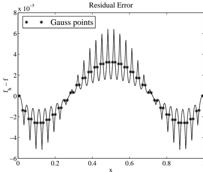
**Fig. 1.** Residual error for 1D Poisson equation.
