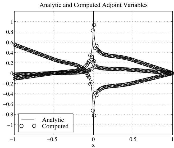
Fig. 7. Adjoint solution for quasi-1D shock-free transonic flow.
