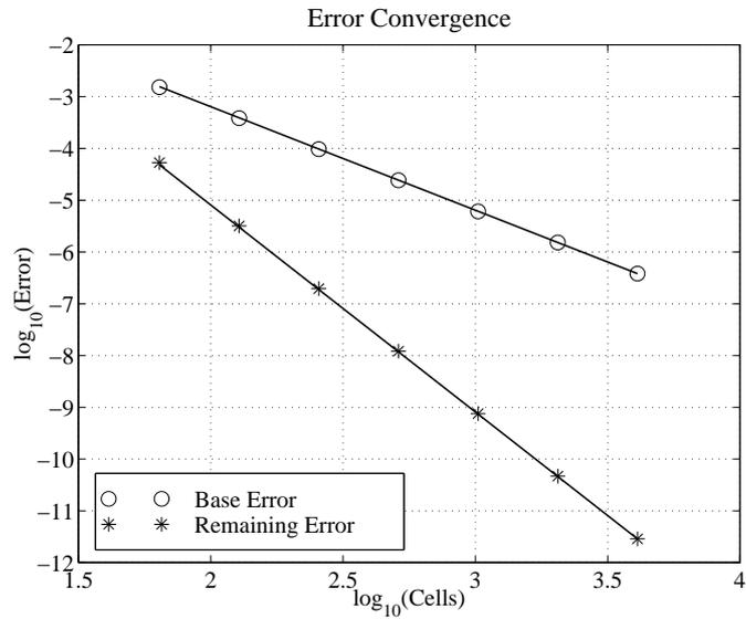
Fig. 6. Error convergence for quasi-1D shock-free transonic flow.
