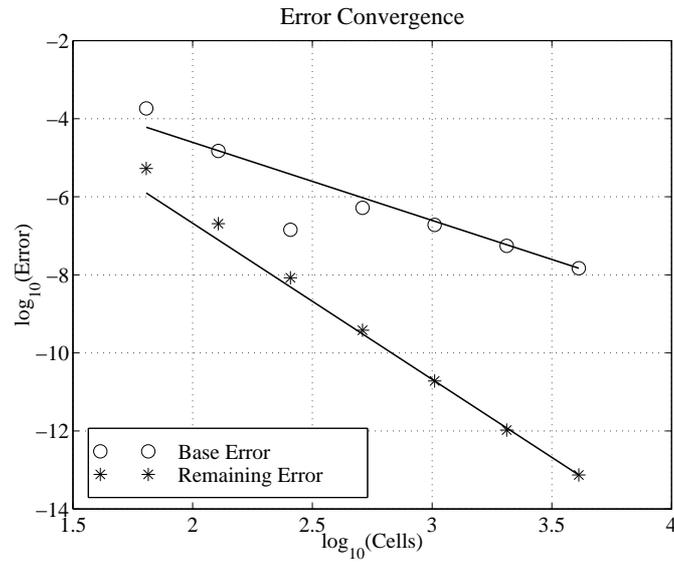
Fig. 5. Error convergence for quasi-1D subsonic flow.
