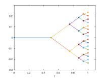
Each path continuation is independent of all of the others, i.e. uses its own Brownian motion. Computational cost per sample is  $O(h_{\ell}^{-1}|\log h_{\ell}|)$ .
