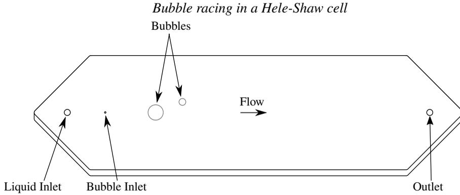
Figure 3: Diagram of the Hele-Shaw cell including bubbles of typical size.
