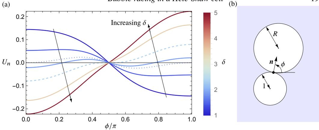
Figure 12: (a) The relative normal velocity,  $U_n$ , of the two bubbles as a function of the polar angle,  $\phi$ , for a fixed  $R = 2$  and  $\delta$  shown by the colour bar. The dotted and dashed curves show  $U_n$  as a function of  $\phi$  at  $\delta = \delta_1(2)$ , and  $\delta = \delta_2(2)$ , respectively (see §5.2). (b) Schematic of two bubbles touching showing the definitions of  $\mathbf{n}$  and  $\phi$ .
