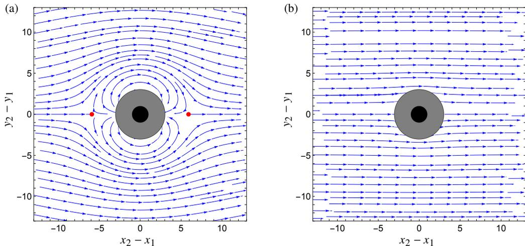
Figure 8: Trajectories for the two-bubble dynamical system (3.17) in the reference frame of the smaller bubble, with  $R = 2$  and (a)  $\delta = 5$ , (b)  $\delta = 1/2$ . Any trajectories entering the solid grey region  $|z_2 - z_1| \leq (1 + R)$  are such that the two bubbles will collide. Stationary points are shown in red. The solid black region  $|z_2 - z_1| \leq 1$  represents the smaller bubble.
