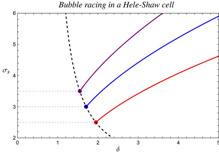
Figure 9: Position of the stationary point,  $\sigma_s$ , as a function of the Bretherton parameter,  $\delta$ , for radius ratios  $R = 1.5$  (red), 2 (blue), 2.5 (purple). The dashed black curve shows where  $\sigma_s = 1 + R$ .
