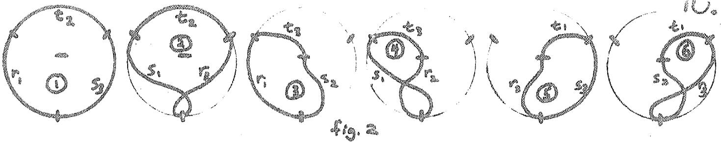
For example, the network in fig. 1 has only six kinds of cycle (shown in fig. 2), all of which are incident (since the bottom bar is common).
