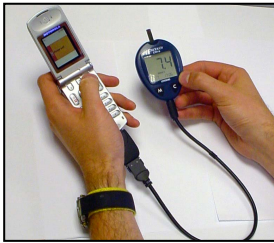
Figure 1. The mobile phone, blood glucose meter and interface cable
