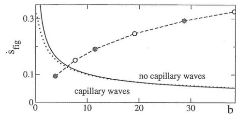
FIG. 3. Transition curves in  $(b, \dot{s}_{\text{fig}})$  parameter space for profiles with and without capillary waves, calculated from the lubrication model (solid line) and Stokes model (dotted line). The dashed line shows the contact-line speed for different slip lengths, calculated from the lubrication model.
