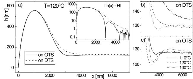
FIG. 2. Rim profiles of 130 nm PS films on DTS and OTS covered Si wafers (a) at constant temperature (the inset depicts a semilog plot of  $|h(x) - H|$ ), (b) and (c) at three different temperatures on DTS and OTS surfaces, respectively. Profiles are shown with the three-phase contact line shifted into the origin.
