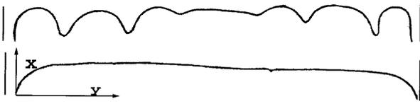
FIG. 2. Top: Film thickness of  $4 \mu\text{m}$ ,  $\tau = 0.19 \text{ Pa}$ ,  $\alpha = 35^\circ$ ; the contact line is almost stable ( $h_\infty = 0.075$ ). Bottom: Film thickness of  $11 \mu\text{m}$ ,  $\tau = 0.11 \text{ Pa}$ ,  $\alpha = 20^\circ$ ; the contact line is stable ( $h_\infty = 0.21$ ). In both cases, the distance between the two vertical bars is  $25 \text{ mm}$ .
