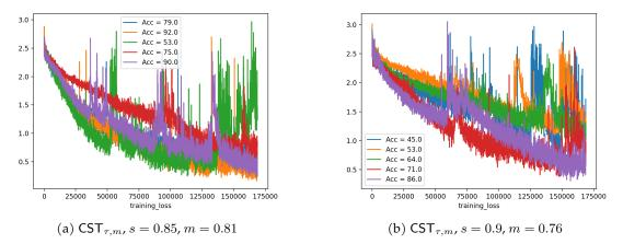
Figure 15: The loss curves during training for each of the 5 runs, for two activation function and hyperparameter configurations with high activation sparsity which achieve low test accuracy as a result of slow and/or unstable training. The legend shows the corresponding final test accuracy achieved by each model.
