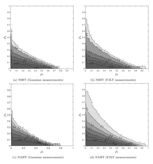
Figure 1: Phase transition level curves denoting the value of  $\delta^*$  for which values of  $\rho_r$  and  $\rho_s$  below which are recovered for at least half of the experiments for  $\delta$ ,  $\rho_r$ , and  $\rho_s$  as given by (140). NIHT is observed to recover matrices of higher ranks and sparsities from FJLT than from Gaussian measurements, while the phase transitions for NIHT and NAHT are comparable. The RPCA projection in NIHT, step 5 in Alg. 1, is performed by AccAltProj [37].
