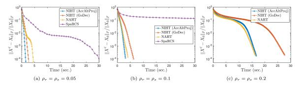
Figure 2: Relative error in the approximate  $X^{\ell}$  as a function of time for synthetic problems with m = n = 100 and  $p = (1/2)100^2$ ,  $\delta = 1/2$ , for Gaussian linear measurements  $\mathcal{A}$ . In (b), SpaRCS converged in 171 sec. (45 iterations), and in (c), SpaRCS did not converge.
