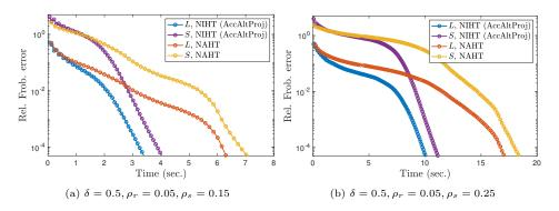
Figure 3: Error between the approximate recovered low-rank and sparse components  $L^{\ell}$  and  $S^{\ell}$  and the true low-rank and sparse components  $L_0$  and  $S_0$ . Error is plotted as a function of recovery time for synthetic problems with m = n = 100 and  $p = (1/2)100^2$ ,  $\delta = 1/2$ , for Gaussian linear measurements  $\mathcal{A}$ .
