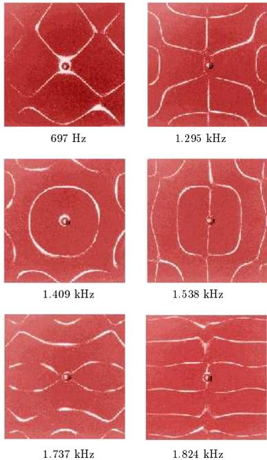
Fig. 1: Chladni figures for a square plate
