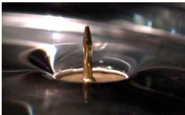
Fig. 3. A photograph of a drawing pin floating upturned on water. Notice that the deformation of the interface in this case is opposite to that around a bubble or near a wetting wall.
