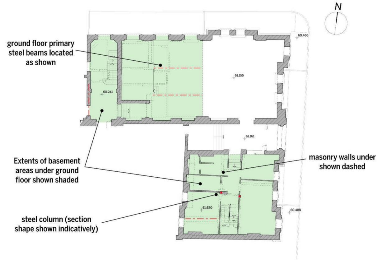
**Figure 4 Ground Floor Structural Arrangement**
