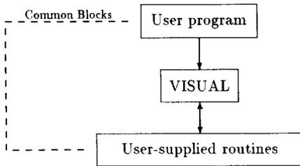
Fig. 1. Flow diagram showing direct use of VISUAL.
