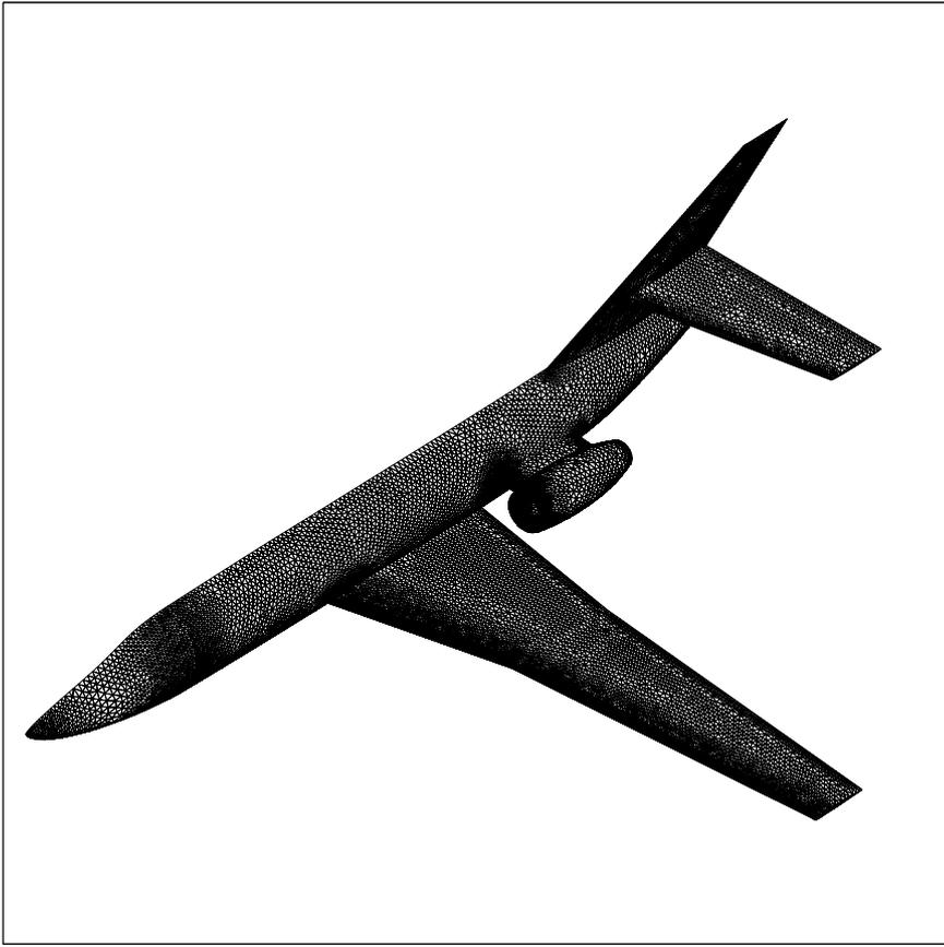
*Figure 2.* Initial surface grid for aircraft wing design (Elliott and Peraire, 1996)
