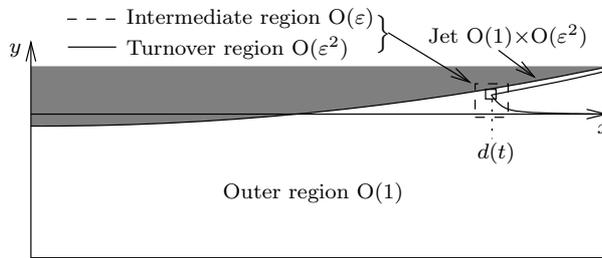
Figure 4: Structure of small deadrise angle impact into a finite-depth layer of fluid.
