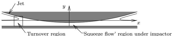
Figure 2: Structure of small deadrise angle impact in the Korobkin flow regime.
