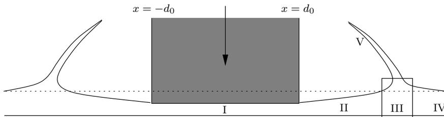
Figure 10: Schematic of zero-deadrise impact in shallow water in the Korobkin flow regime.
