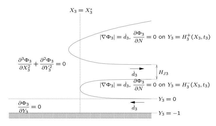
The position of the stagnation point(s) is important. For small times there is one stagnation point, in the fluid. However at a finite time it *touches down* on the base. After this, there are two stagnation points on the wall.
