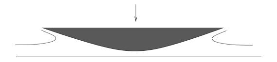
In this talk we deal with the impact of a liquid drop on a thin layer of liquid. The motivation is from models of icing of aircraft. The assumptions are as above: inviscid irrotational flow, no gravity, surface tension, viscosity or compressibility.
