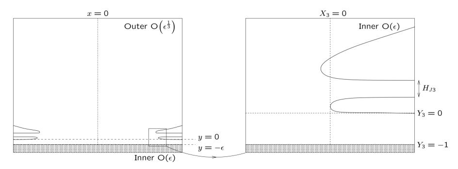
The outer problem is still a Wagner problem of a drop hitting a solid base. In the intermediate stage the drop switches from feeling a liquid layer to feeling only the base (to leading order) but the jet is still unaffected by the base.
