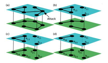
Figure 3.2: The cascade process on coupled networks. Panel (a) shows the initial failure of a node, and the removal of the edges connected to the node. Panel (b) shows the  $a_1$ -clusters, as described in step 1. Panel (c) shows the state of the coupled networks after step 2, and panel (d) shows the state of the networks when the cascade process terminates (step 4). This figure is adapted, with permission, from Fig. 7 in [19].
