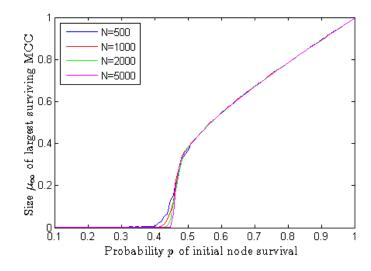
Figure 5.4: Simulations of the cascade process for an attack targeted by 2degree on coupled Erdős-Rényi networks, with mean degrees a = b = 6. 100 simulations were carried out for N = 500, 50 for N = 1000, and 20 each for N = 2000 and N = 5000.
