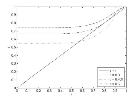
Figure 3.4: A graphical solution to Eq. (3.14), for coupled Erdős-Rényi networks with equal mean degrees (a = b = 6). We plot the curve  $y = \exp\left[-p(r^a - 1)^2\right]$  for p = 0.3, 0.409, and 0.6; and we consider the points of intersection with the line y = r.
