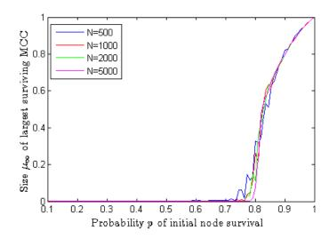
Figure 4.5: Simulations of the cascade process for coupled scale-free networks. All curves are averages of 20 simulations.
