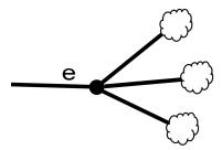
Figure 3.3: The cluster reachable by following a random edge e. In this example, e has excess degree 3. The bubbles represent the clusters reached by following each of the three edges.
