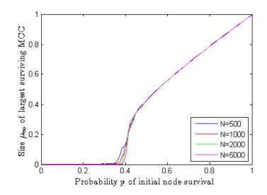
Figure 3.5: Simulations of the cascade process for coupled Erdős-Rényi networks with equal mean degree, a = b = 6. The size of the largest surviving mutually connected cluster is given as a fraction  $\mu_{\infty}$  of the size of the full network. The curves plotted are averages, taken over 50 simulations.
