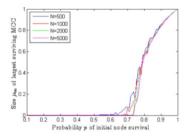
Figure 5.5: Simulations of the cascade process for an attack targeted by 2-degree on coupled scale-free networks. All curves are averages over 20 simulations.
