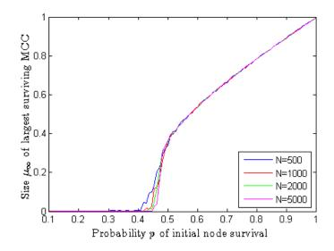
Figure 4.4: Simulations of the cascade process for an attack targeted by node degree on coupled Erdős-Rényi networks with equal mean degree (a = b = 6). All curves are averages of 20 simulations.
