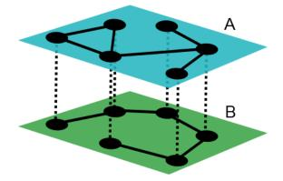
Figure 3.1: An example of coupled networks. Edges within networks are represented by solid lines, and dependencies between networks are represented by dotted lines. A-edges join nodes in A and B-edges join nodes in B. Each node in A depends on, and is depended upon by, exactly one node in B. This figure is adapted, with permission, from Figure 7 in [19], using Inkscape ([17]).
