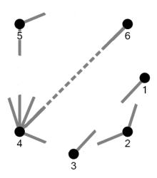
Figure 2.1: Illustration of the formation process for the configuration model. This example generates a random graph with degree sequence (1,2,1,5,2,1). The dotted line shows a pair of edges that has been chosen uniformly at random, and joined to each other. This figure was created using the NodeXL template for Microsoft Excel ([25]).
