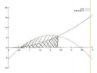
$$\int_{\frac{6-\sqrt{12}}{4}}^{\frac{6+\sqrt{12}}{4}} \left(6-3(x-2)^2\right) dx - \int_{\frac{6-\sqrt{12}}{4}}^{\frac{6+\sqrt{12}}{4}} x^2 dx = \int_{\frac{6-\sqrt{12}}{4}}^{\frac{6+\sqrt{12}}{4}} \left(6-3(x-2)^2-x^2\right) dx$$
