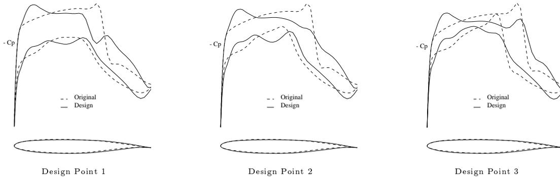
Figure 6: Multipoint drag minimization at fixed lift. Pressure distributions at the  $z=0.475$  span station for the three design points described in Table 2 [41].
