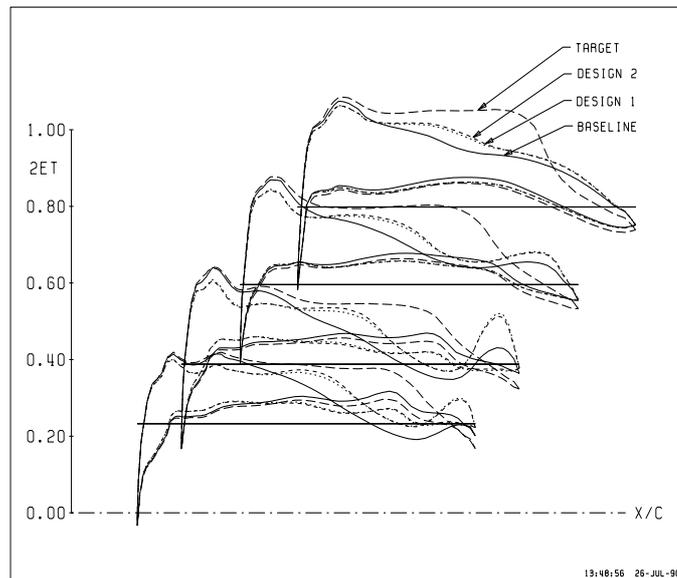
Figure 4: Evolution of the pressure distribution on the wing [10]
