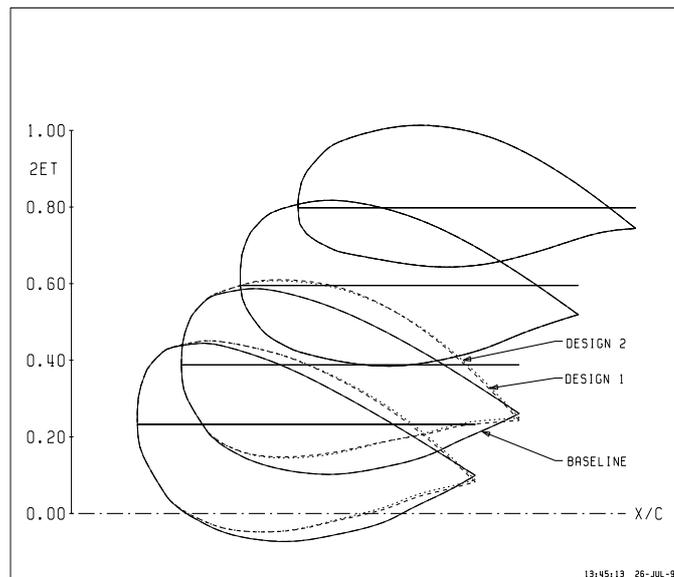
Figure 3: Evolution of the wing geometry during design [10]
