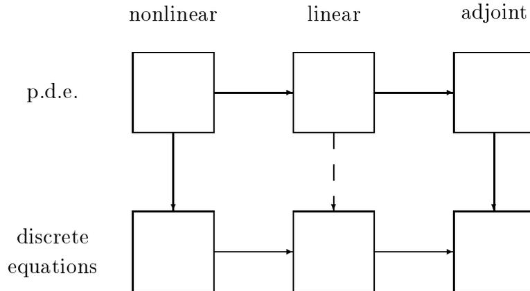
Figure 1: Alternative approaches to forming discrete adjoint equations
