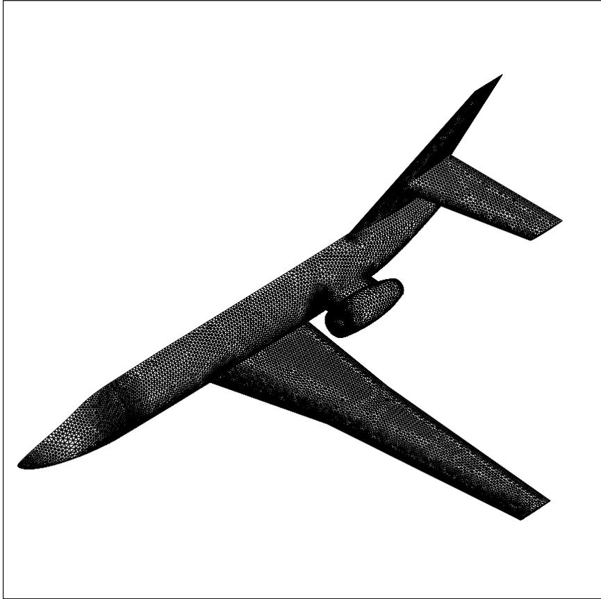
Figure 2: Initial surface grid for aircraft wing design [10]
