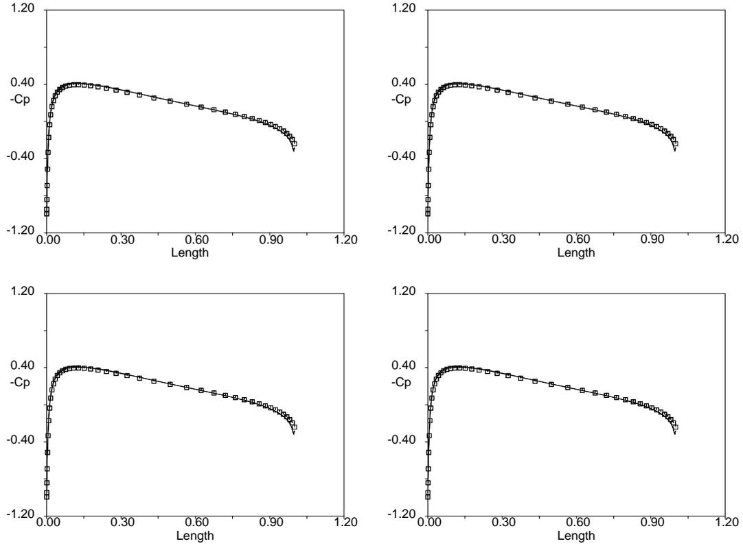
Figure 4: Computed pressure coefficient contours around a Naca0012 airfoil. Comparison with the potential flow solution.  $M_\infty = 0.1, 0.01, 0.001, 0.0001$ .  $\alpha = 0^\circ$ .
