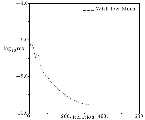
Figure 7: Convergence history comparison for a low Mach number flow over the M6 wing. Viscous calculation.  $M = 0.1$ ,  $\alpha = 0^\circ$ ,  $Re = 3 \times 10^6$ .
