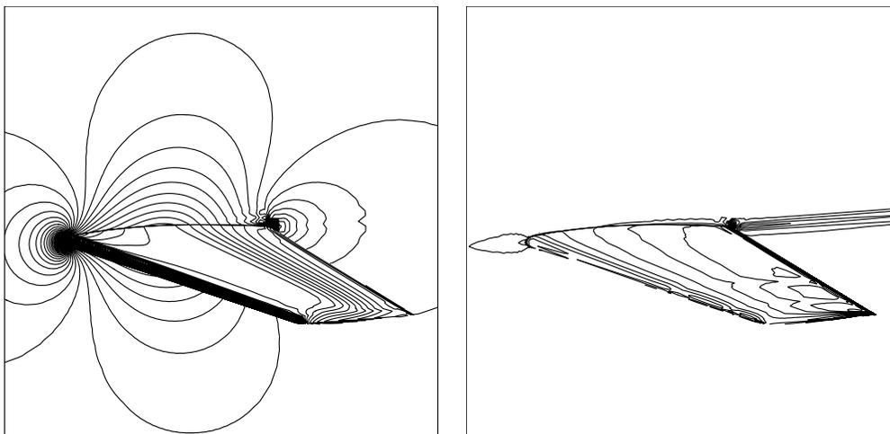
Figure 6: Inviscid flow over the M6 wing: computed pressure plot for  $M_\infty = 0.0001$  with and without low Mach number preconditioner.  $\alpha = 0^\circ$ .
