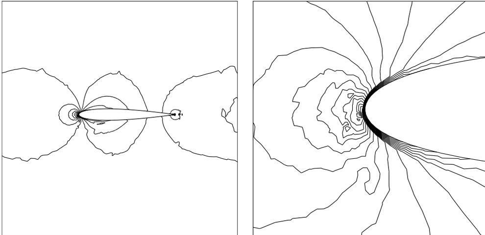
Figure 1: Computed pressure plot for  $M_\infty = 0.01$  without low Mach number preconditioner.  $\alpha = 0^\circ$ .
