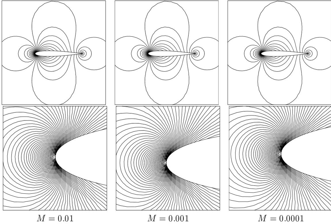
Figure 2: Computed pressure coefficient contours around a Naca0012 airfoil, overview and zoom around the leading edge.  $\alpha = 0^\circ$ .
