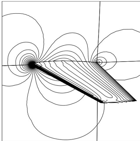
Figure 8: Viscous flow over the M6 wing: computed pressure plot for  $M_\infty = 0.1$  with low Mach number preconditioner.  $\alpha = 2^\circ$ ,  $Re = 3 \times 10^6$ .
