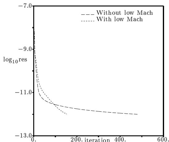
Figure 5: Convergence history comparison for a low Mach number flow over the M6 wing. Inviscid calculation.  $M = 0.0001$ ,  $\alpha = 0^\circ$ .
