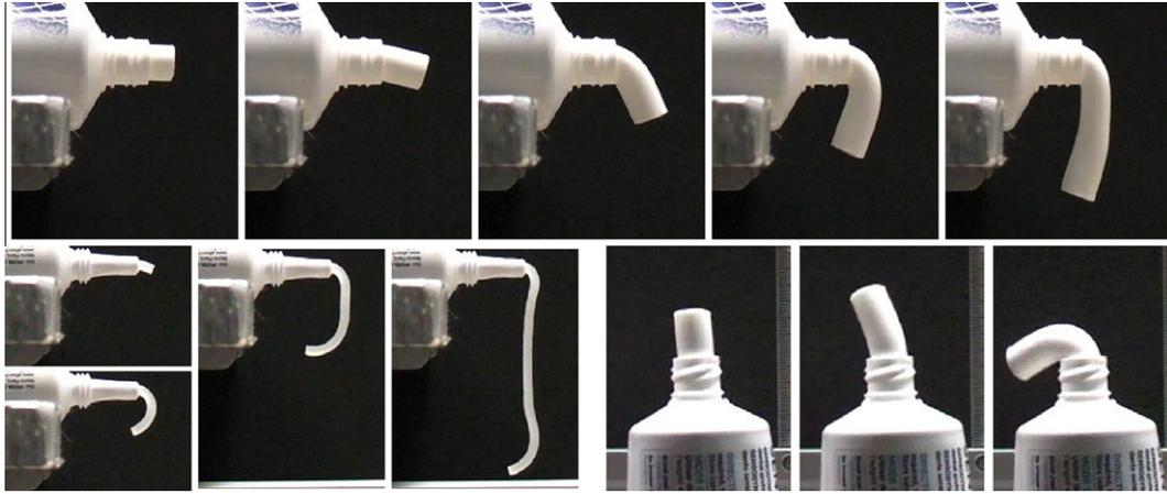
**Fig. 1.** Top row: a horizontal extrusion of “Sensodyne Whitening” toothpaste. The photographs are four seconds apart. Lower left: an extrusion of “Neosporin” (images are 2, 2 and 3 seconds apart). Lower right: extruding the Sensodyne toothpaste vertically, with images 1 and 0.5 seconds apart.
