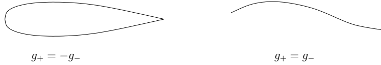
Figure 4.7: Schematic of a symmetric aerofoil (left); a zero-thickness aerofoil (right).
