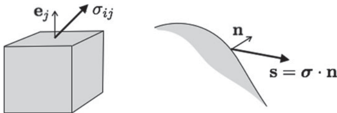
Fig. 1.3 The stress acting on the j th face of a cube, and on an arbitrary surface with unit normal \mathbf{n}
