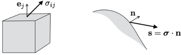
Figure 3: The stress acting on the j th face of a cube, and on an arbitrary surface with unit normal \mathbf{n}
