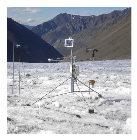
A weather station on the ice surface measures atmospheric properties in a (roughly) Eulerian framework.
