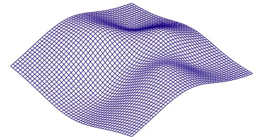
Fig. 2: A thin-plate spline, interpolating function values given at 9 scattered points
