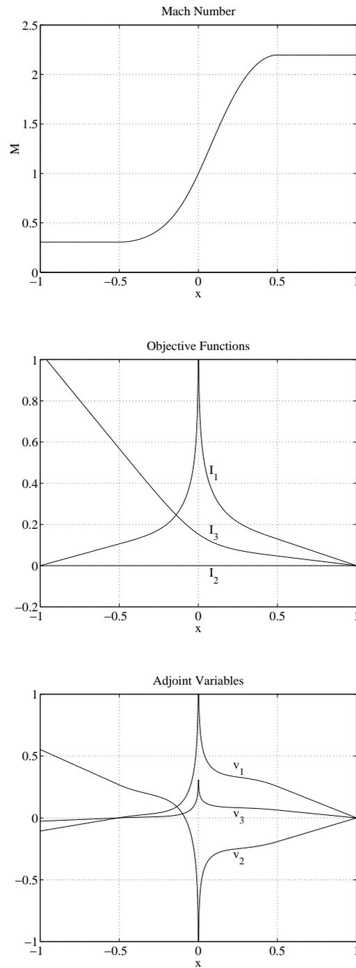
Figure 3: Mach number, objective functions and adjoint variables for isentropic transonic flow conditions.  $H_{\text{in}} = 4, p_{0\text{in}} = 2$ .
