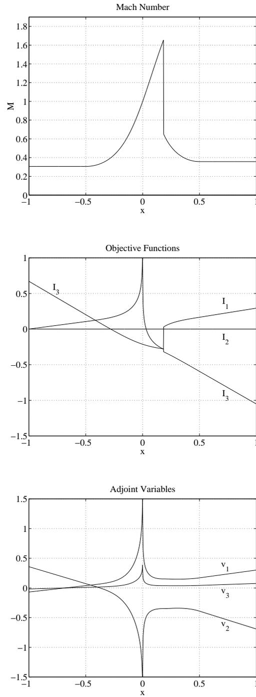
Figure 4: Mach number, objective functions and adjoint variables for shocked flow conditions.  $H_{\text{in}} = 4$ ,  $p_{0\text{in}} = 2$ ,  $p_{\text{ex}} = 1.6$ .
