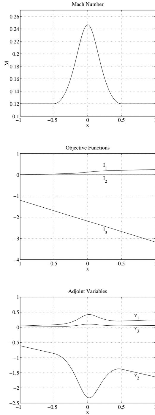
Figure 2: Mach number, objective functions and adjoint variables for subsonic flow conditions.  $H_{in} = 4$ ,  $p_{0in} = 2$ ,  $p_{ex} = 1.98$ .
