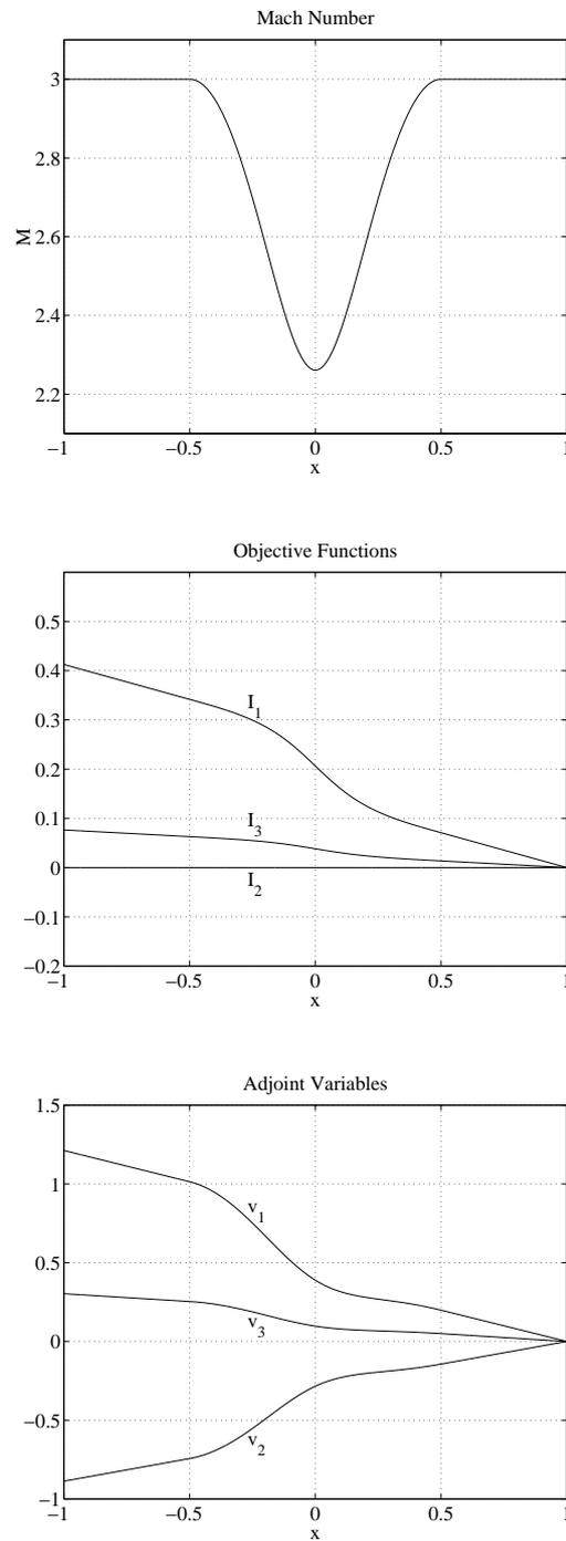
Figure 1: Mach number, objective functions and adjoint variables for supersonic flow conditions.  $M_{\text{in}} = 3$ ,  $H_{\text{in}} = 4$ ,  $p_{0\text{in}} = 2$ .
