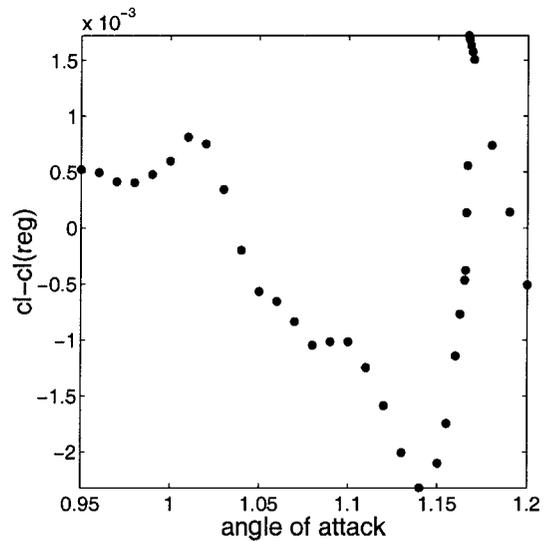
Fig. 6  $C_l - C_l(\text{regression})$  for NACA 0012 at  $M = 0.85$ .
