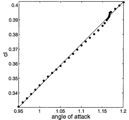
Fig. 5  $C_l$  vs angle of attack for NACA 0012 at  $M = 0.85$ .
