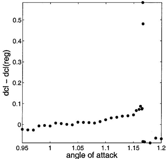
Fig. 7 NACA 0012 at  $M=0.85$ ,  $dC_l/d\alpha(\text{linear}) - dC_l/d\alpha(\text{regression})$ .
