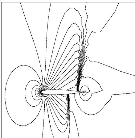
Fig. 4 Mach contours for NACA 0012 at  $M = 0.85$ .
