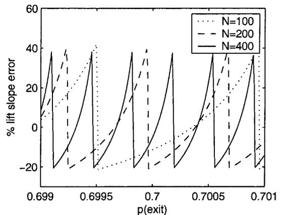
Fig. 11 Lift slope error for quasi-one-dimensional test case with uniform grid spacing  $\Delta x = 1/N$ .
