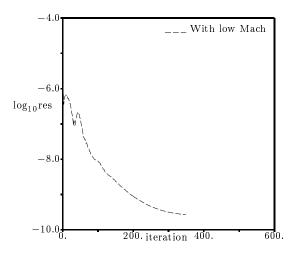
Figure 7: Convergence history comparison for a low Mach number flow over the M6 wing. Viscous calculation. M = 0.1,  $\alpha = 0^{o}$ ,  $Re = 3 \times 10^{6}$ .
