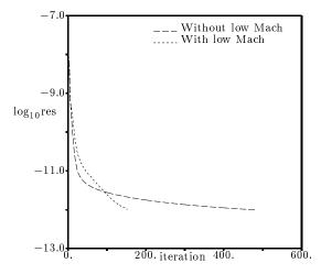
Figure 5: Convergence history comparison for a low Mach number flow over the M6 wing. Inviscid calculation. M = 0.0001,  $\alpha = 0^{\circ}$ .
