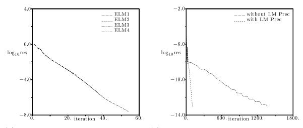
(a) Tests ELM1, ELM2, ELM3, ELM4.(b) Low Mach number preconditioner effect.Figure 3: Convergence history comparison for low Mach number flow around a Naca0012 airfoil.
