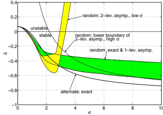
Figure 4. Aeroelastic stability with random mistuning; exact and asymptotic analyses with Monte Carlo simulations
