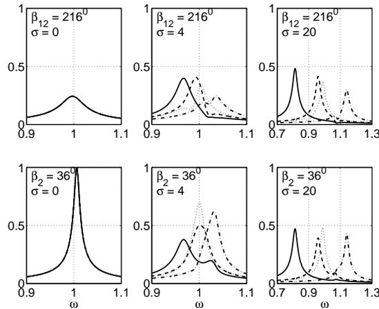
Figure 6. Blade response of randomly mistuned assembly for two engine orders and for different levels of mistuning. (—: blade 7, ---: blade 19, ...: blade 13, -.-.: blade 10)
