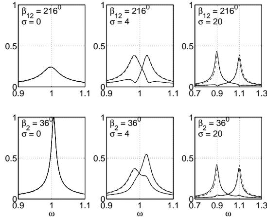
Figure 5. Blade response of alternately mistuned assembly for two engine orders and for different levels of mistuning. (—: exact, ---: asymptotic)
