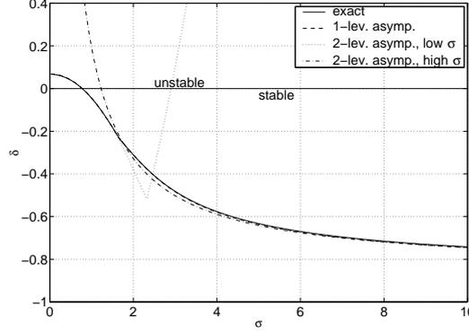
Figure 2. Aeroelastic stability with alternate mistuning. Exact and asymptotic analyses
