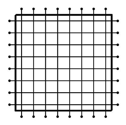
Each block of threads will work with one of these grid blocks, reading in old values (including the "halo nodes" from adjacent partitions) then computing and writing out new values
